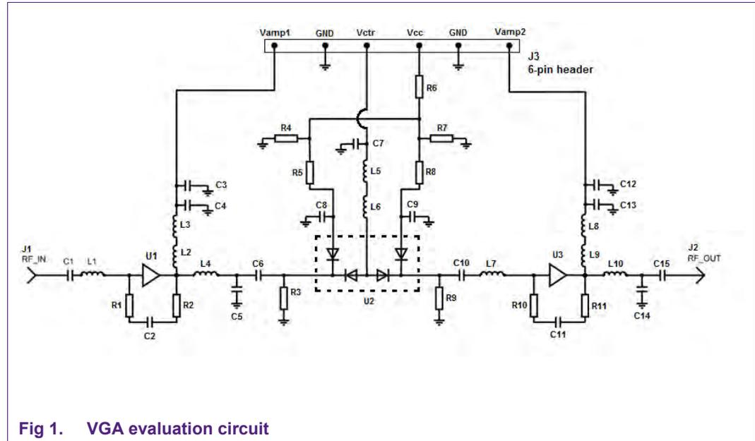
Fig 1. VGA evaluation circuit
