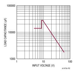
Figure 2. Maximum Permissible Load Capacitance at Start-Up
