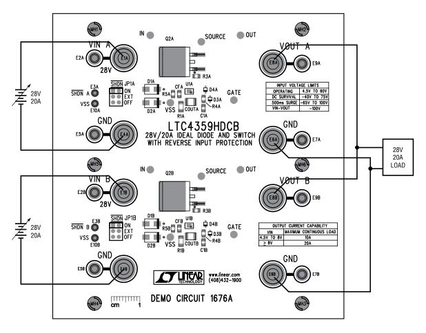
Figure 5. Basic Test Setup
