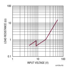
Figure 3. Minimum Permissible Load Resistance at Start-Up
