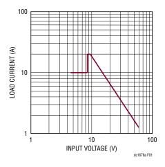
Figure 1. Maximum Permissible Constant Current Load at Start-Up
