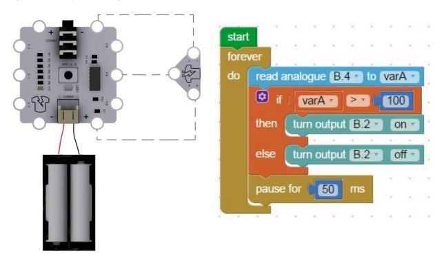
The positive and negative terminals of the Light Level Detector are connected to the positive and negative supply pins of the Igloo. The OUT pin of the Light level detector is connected to an analogue input pin of the Igloo. The code then reads the analogue value and uses it to make a decision to turn the output on or off.
