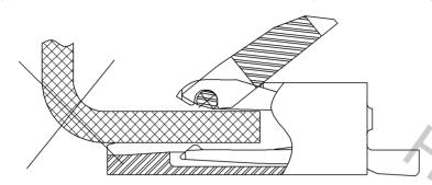
5. Do not rotate the actuator when FPC TAB is on Metal Fittings.
