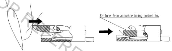
The actuator is designed to rotate on the axis shown in the figure below so make sure to use a rotating motion when operating it.
