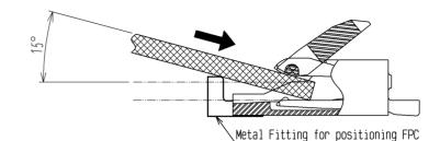
2. When inserting the FPC, make sure not to bump the FPC's tip against the upper arm area of the terminal. This may cause the terminal to deform.
